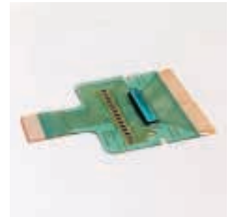
In April 2003 Toyo Metallizing Co. brought new capacity on stream for manufacturing Metaloyal ® , a flexible material for high-density electronic circuits formed on copper electroplated polyimide film.
