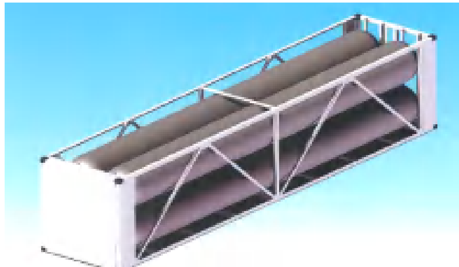
Tube trailer tank (length 12 m)
