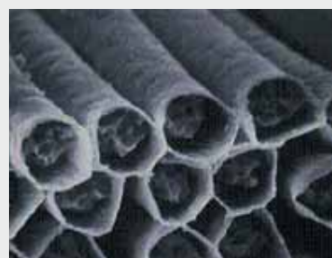
Cross-section of a functional material-coated fibers using NanoMATRIX* technology
