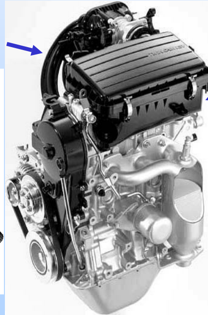
Intake Manifold (Nylon6 GF30)
