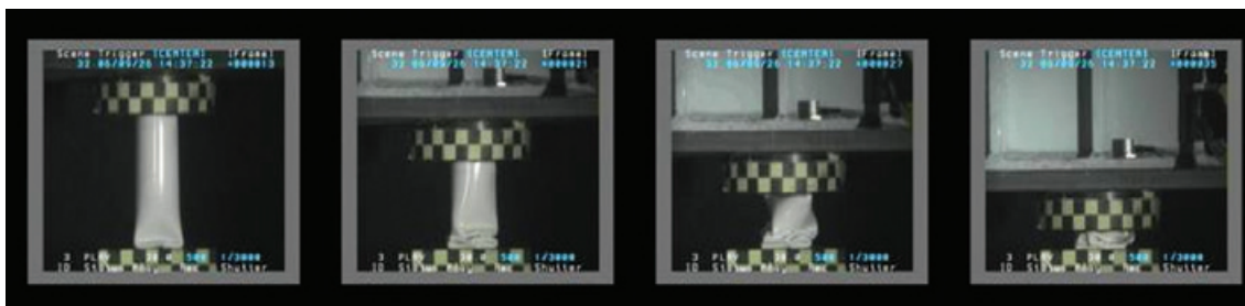
Change shape flexibly and absorb the impact-energy
