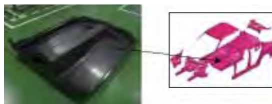
The front floor of a platform formed in ten-minute molding cycle
