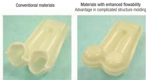
\*Comparison with model-molded products (glass fiber reinforced nylon 6, special polymer 1 wt% added)
