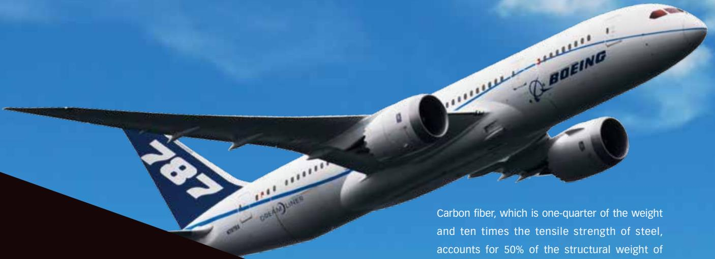
Carbon fiber, which is one-quarter of the weight and ten times the tensile strength of steel, accounts for 50% of the structural weight of Boeing 787s. The environmental impact of aircraft is drastically reduced by making them lighter.
