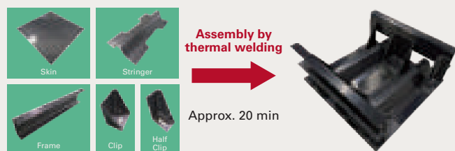
Thermally Welded Assembly of Aircraft Structural Demonstrator Applying this Technology
