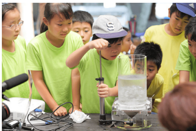
Testing the moisture-permeable waterproof qualities of ENTRANT™ fabric, which breathes air delivered from beneath while remaining impermeable to the cylinder of water on top of the fabric
