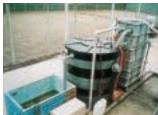
Toray Monofilament Co., Ltd. Membrane bioreactor (MBR) Pilot system
