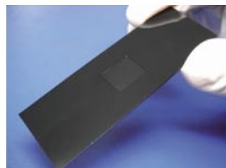
Ultrasensitive DNA Chip for the detection of pollutant-degrading microorganisms
