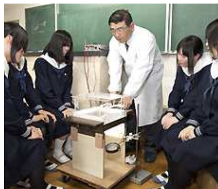
One of the awarded works was a device that observes the propagation of waves. By using an LED to light two circular wave patterns from below the water's surface, ripples are projected and enlarged onto the ceiling.
