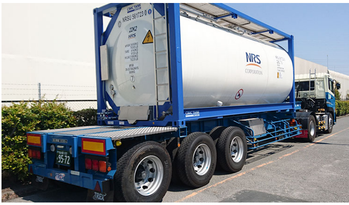
ISO-specification tank container and transport chassis
