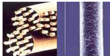
Left photo: Cross-sectional view of uniform ultrafine fibers produced by sea-island conjugate spinning (image) Right photo: The diameter of the ultrafine fiber developed by Toray (left in the photo) is 1/50 of a hair (right in the photo).
