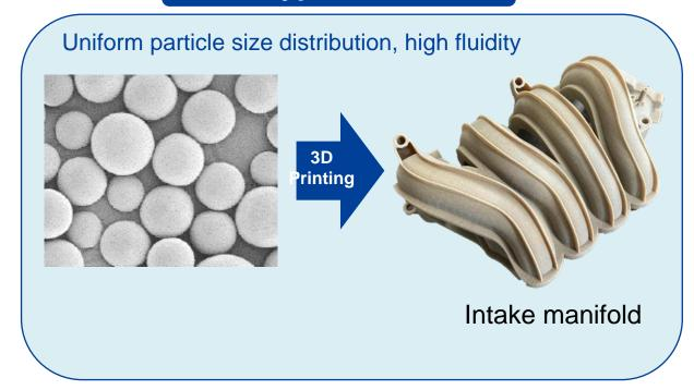
No machining wastes and mold-free, reduction of inventory (parts) through on-demand production →Realization of sustainable manufacturing
