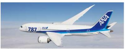
A totally carbon fuselage was achieved for the Boeing 787. CFRP was used as the primary structural material for the main wings, tail, and fuselage of the aircraft, and accounts for about 50% of the weight of the structural elements. (Photograph courtesy of All Nippon Airways Co., Ltd.)
