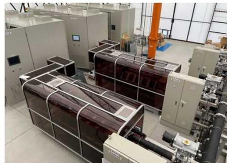
2.3MW class PEM type electrolyzer demonstration machine (in collaboration with Hitachi Zosen Corporation)
