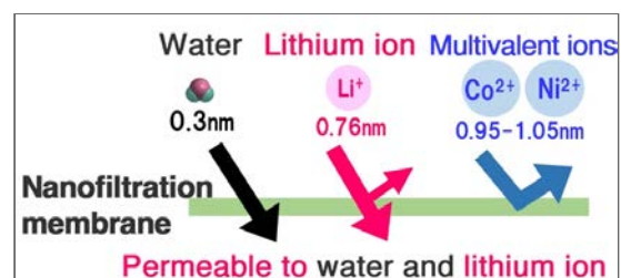
Lithium separation using nanofiltration membranes
