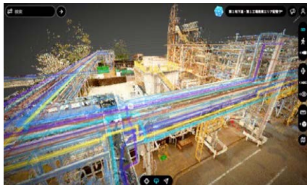
Functions of various pipelines are made clear on the computer screen using 18 different colors
