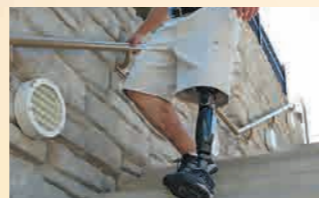
義足用炭素繊維複合材料 Carbon fiber composite materials for prosthetic legs
