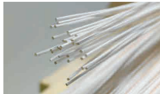
独自の熱誘起相分離法による強靱さと精密細孔を併せ持つPVDF中空糸膜 PVDF hollow fiber membranes featuring both toughness and a precise pore structure due to our unique thermally induced phase separation method
